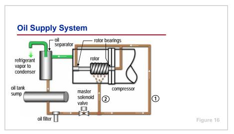
Oil that collects in the oil sump is at condensing pressure during compressor
